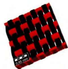
Fig. 1. Reinforcement microstructure of a carbon fiber composite laminate modelled with
