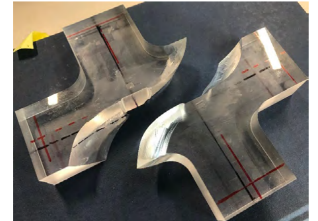
Figure 5. PMMA biaxial specimen - post fracture
