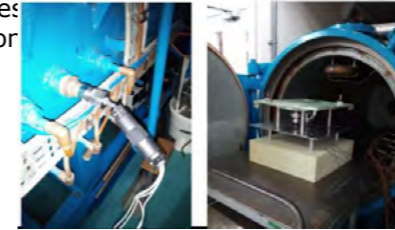
Fig.2. Autoclave setup with US transducers
