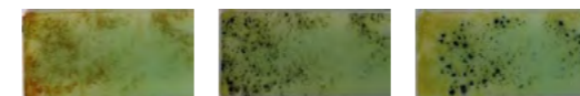
Figure 4 TB and epoxy powder coated glass immersed in 0.1M of NaOH for: 0 days (left), 2 days (centre) and 35 days (right).
