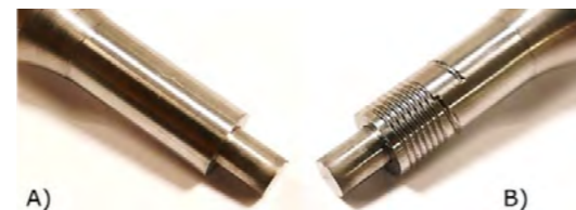
Figure 2 - M42 RFSSW tools components: A) Tool 2 and B) Tool 3.
