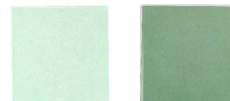
Figure 7 phph and epoxy powder coated TSZA S355 plates exposed to seawater for: 0 days left, and 35 days (right)
