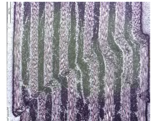
Figure 3. Optical microscope image of a pierced coupon tested under OHC loading.
