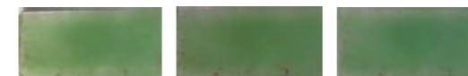
Figure 3 phph and epoxy powder coated glass immersed in 0.1M of NaOH for: 0 days (left), 2 days (centre) and 35 days (right).
