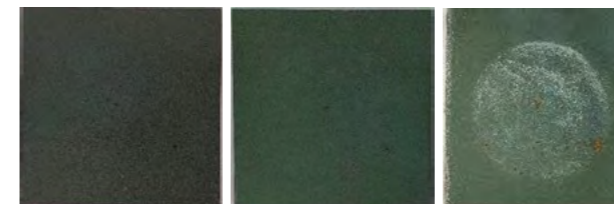
Figure 5 phph and epoxy powder coated S355 plates exposed to seawater for: 0 days (left), 7 days (centre) and 35 days (right).
